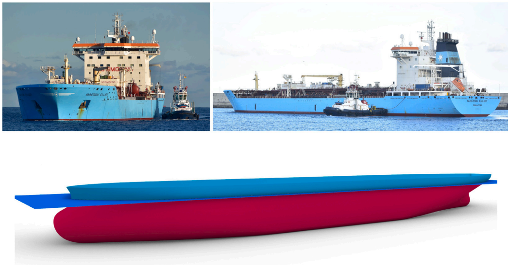
Fig. 4. Typical tankers are landing in the port of Koper, where C_B \approx 0.8 . The authors created a CAD model in Rhino3D based on the technical construction documentation of a geometrically identical tanker to determine hydrodynamic coefficients.
